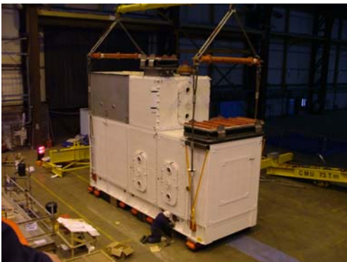
Set Down to temporary support blocks prior to road haulage
